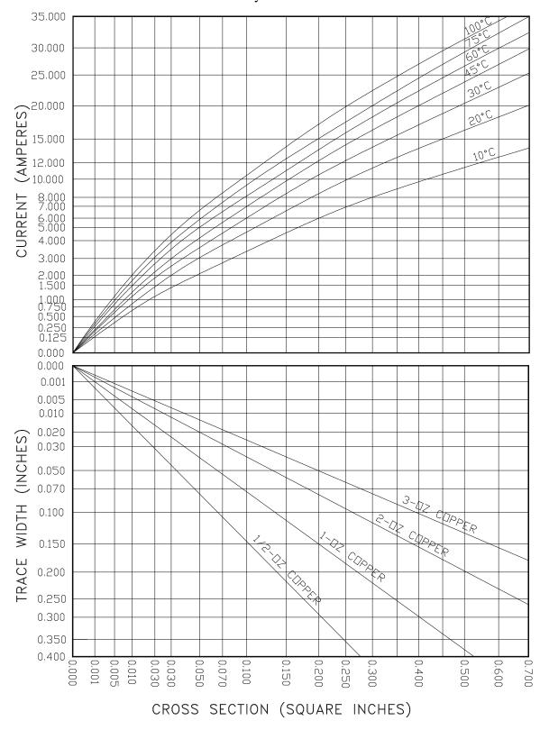
For use in determining current carrying capacity and size of etched copper conductors for various temperature rise above ambient.
