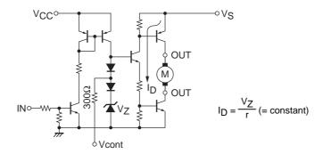
As shown in the above diagram, the Vcont pin outputs the voltage of the band gap Zener  $V_Z + V_F$  (=1.93V). In normal use, this pin is left open.
