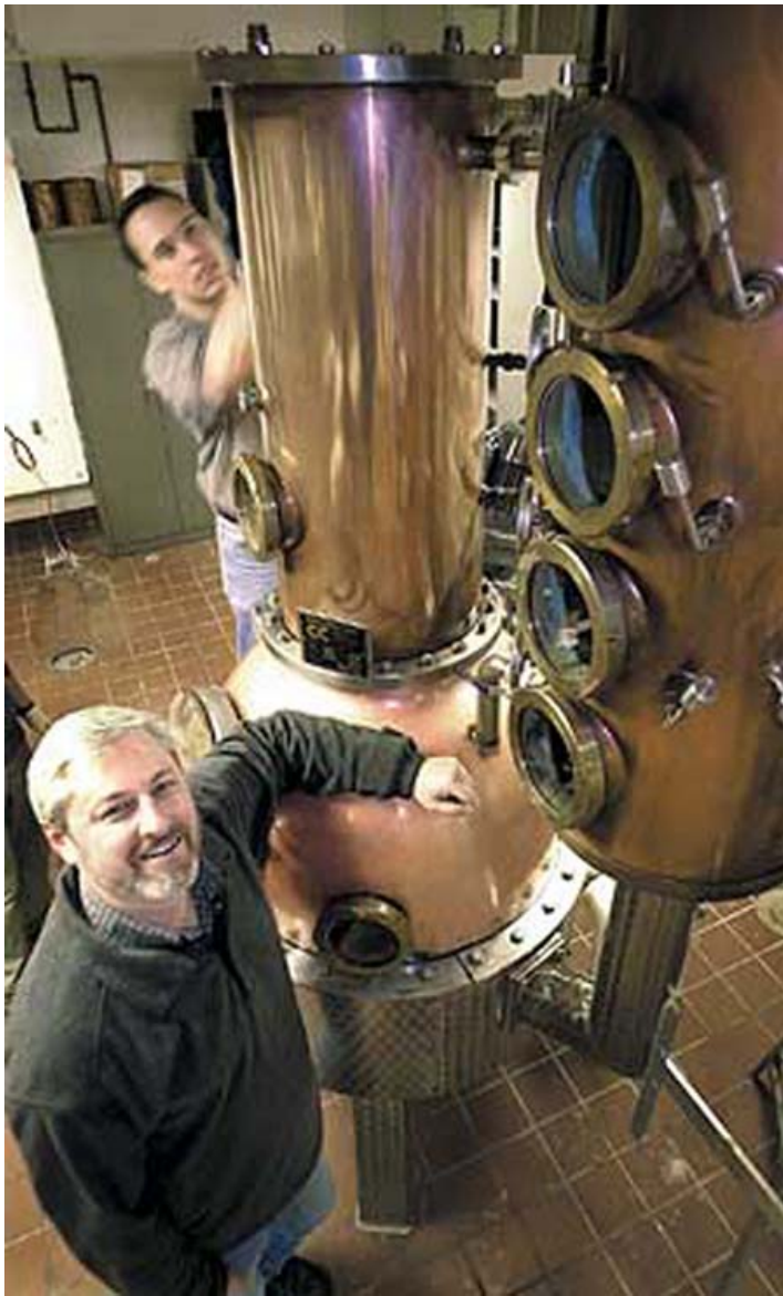
The author (KAB) in the foreground with former MSU graduate student, Matt Berg, in the background at the MSU distillery in East Lansing, MI USA. This 150 liter working volume still is a typical still used by the artisan distillers in Michigan.
