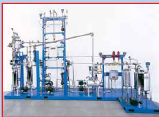
Skid-Mounted Purification Plant , with 2" diameter fractionating column, reboiler, condenser, vaporizers, pumps, control elements, vessels and other components.
