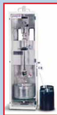
Pope Hybrid Distillation System , incorporating 12" diameter fractionating column with 10 square foot wiped-film evaporator for purification of heat-sensitive compounds. System also incorporates Molecular Still and explosion-proof control system.
