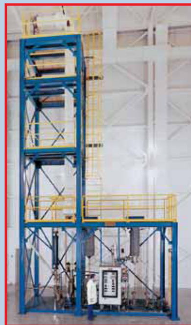
Pope Hybrid Distillation System , incorporating 12" diameter fractionating column with 10 square foot wiped-film evaporator for purification of heat-sensitive compounds. System also incorporates Molecular Still and explosion-proof control system.
