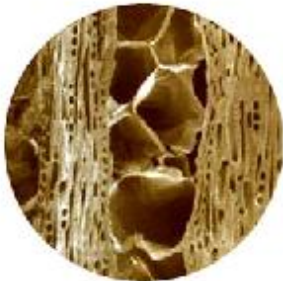
Photo-micro graph. Oak has through-capillaries, is micro-porous to gases.
