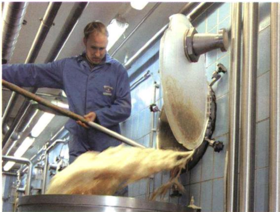
A lay worker at Westmalle (above) top crops yeast. The brewery installed a state-of-the-art bottling line (below) in 1999.
