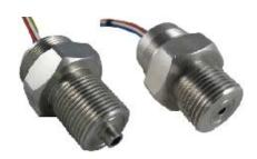
HR-PT11 industrial pressure sensor is a standard and most popular sensor applied in air and liquid pressure measuring. A high sensitivity silicon pressure chip is employed in the transducer. The sensor is welded with the housing, no leakage will happen. It is more reliable compared with O-ring sealing for leakage.
