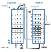
The wash is pumped in at the top of the rectifier where, as it flows down a coil, it is warmed by the heat of vapours rising up the still. Once heated, the wash enters the top of the analyser.
