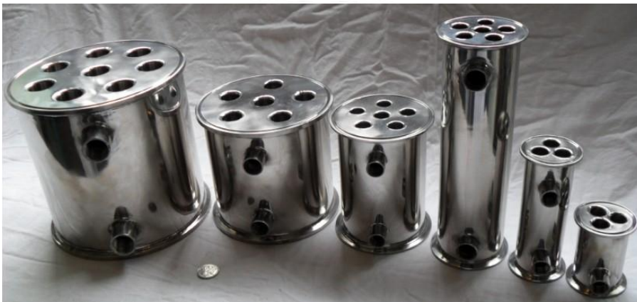
Figure 30: Various Size Dephlegmators (Reflux Condensers)
