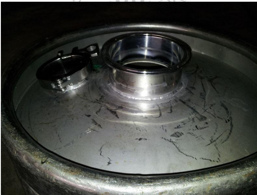
Figure 4: A 4" Ferrule welded onto what was the bottom of a keg. A fill port can also be seen.
