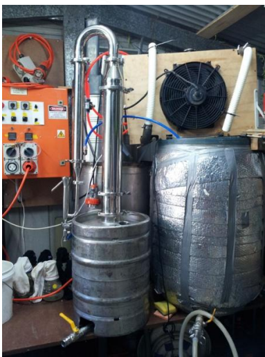
Figure 18: The Authors 4" Pot Still using a 510mm Extension
