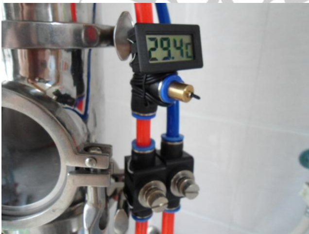
Figure 42: Connect Needle Valves & Thermo Tee's where they are Easy to Reach
