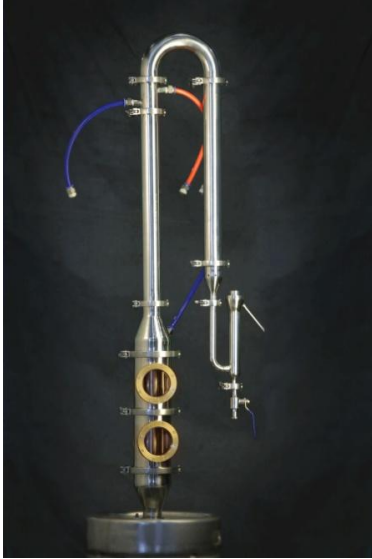
Figure 27 2 Plates with a 2" Packed Section
