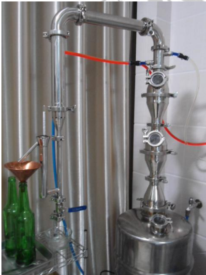
Figure 22: A 2 Plater using Torpedos
