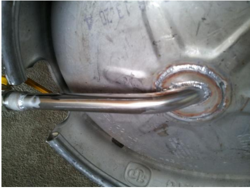
Figure 3: Low Profile Drain on what was the top of the keg
