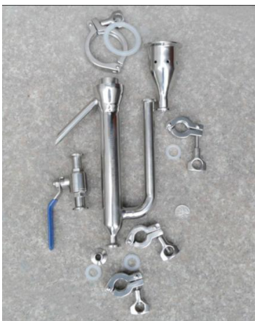
Figure 14: A Disassembled Parrot - As Shipped
