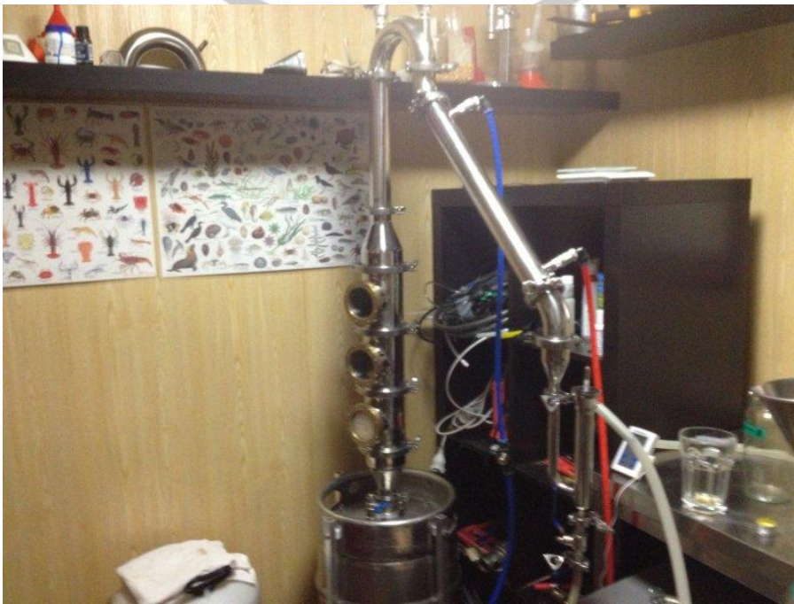
Figure 20: Bubble Tee's Being Run Without Plates
