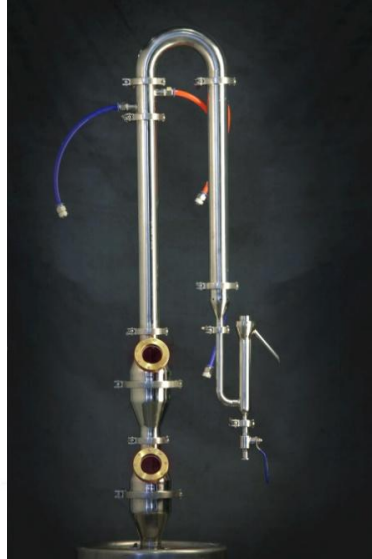
Figure 28 2 Torpedos with a 2" Packed Section
