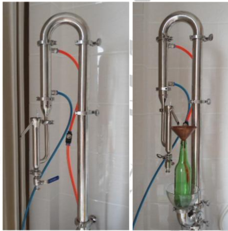
Figure 17: 2" pot stills made from extensions
