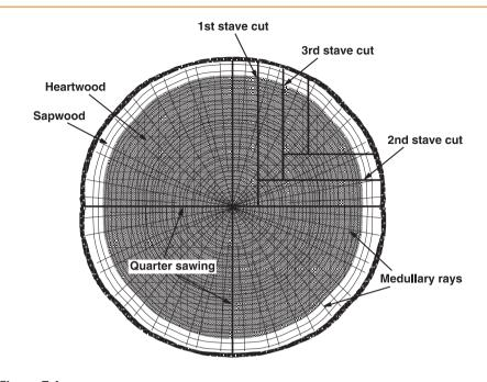
Figure 7.1 Stave cuts in timber processing.
