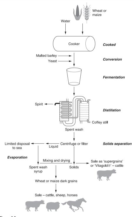
Figure 8.2 Grain distilling co-products – typical process.
