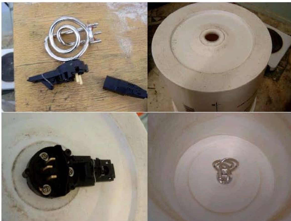
PIC – boiler and heating element
