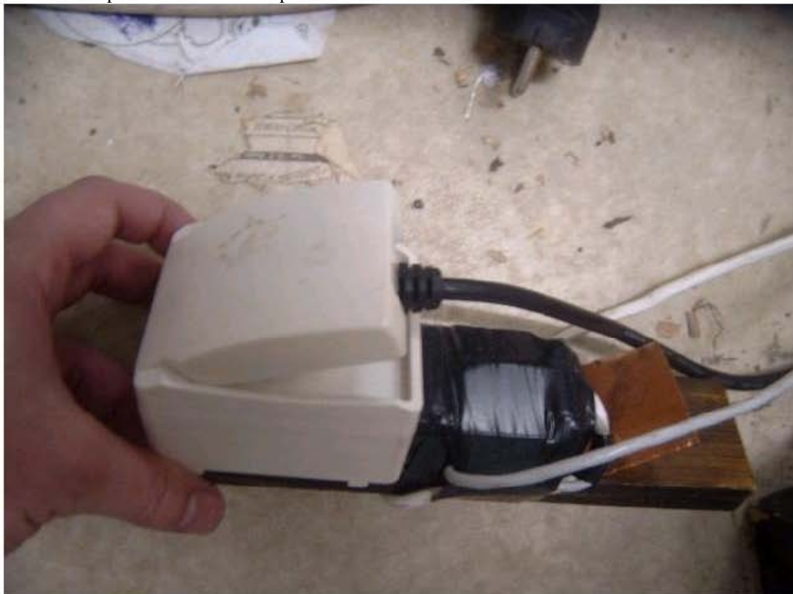
PIC – power controller system, relay under the black tape
