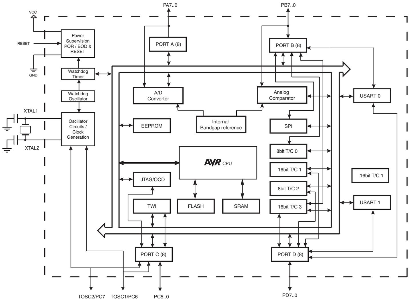
The AVR core combines a rich instruction set with 32 general purpose working registers. All the 32 registers are directly connected to the Arithmetic Logic Unit (ALU), allowing two independent registers to be accessed in one single instruction executed in one clock cycle. The resulting architecture is more code efficient while achieving throughputs up to ten times faster than conventional CISC microcontrollers.
