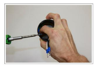
3. Unscrew the bolts from the element. Attach the positive and negative leads to the bolts and re-attach to the element. Ensure that the leads are not contacting the enclosure sides. Polarity is unimportant.
