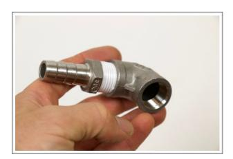
7. Slip the red silicone washer over the stainless nipple and push the nipple of the tee assembly through the hole on the lid. From the underneath of the lid screw the 90° stainless elbow to the nipple. Use two wrenches to tighten.
