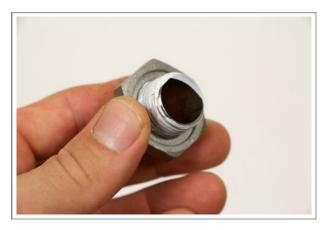
3. Thread the pipe nipple into the tee as show, with the groove facing away from the tee fitting. Finger tighten only.
