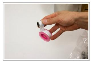
2. Thread the 1/2" locknut onto the pipe nipple until it stops at the centre. Ensure that the groove in the locknut is facing towards the centre of the pipe nipple.
