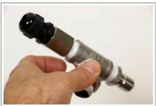
6. Wrap the 1/2" MPT barb fitting with 4 wraps of teflon tape. Screw the MPT barb fitting into the 90° stainless elbow and tighten with 2 wrenches.
