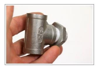
4. Wrap the Male/MPT quick disconnect with 4 wraps of teflon tape and screw into the tee as shown. Use 2 wrenches to tighten.
