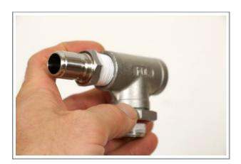
5. Depending on your temperature controller used, wrap either the RTD sensor threads, or the stainless thermowell threads with 4 wraps of teflon tape and screw into the tee as shown. Use 2 wrenches to tighten. Screw the sensor strain relief in to the thermowell.
