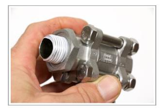
4. Wrap the male-to-MPT quick disconnect with 4 layers of teflon tape and thread it into the other end of the ball valve. Tighten the ball valve to the QD fitting using 2 wrenches.
