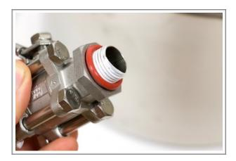
6. Position the nipple into the cutout of the pot and slide the 1" washer over the nipple. Thread the 1/2" coupling on and finger-tighten it. Using two wrenches, tighten the coupling and the ball valve until they are tight to the pot.
