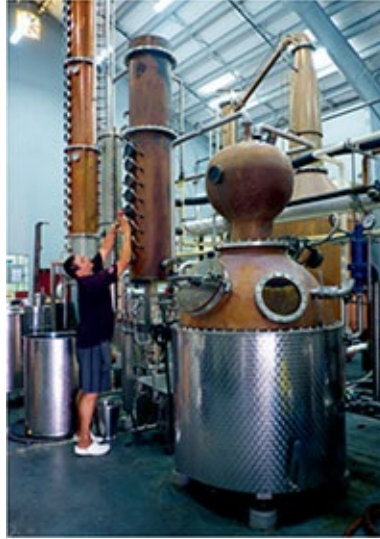
At the back right is the Vendome stripping still, and in the front is the Christian Carl pot.
