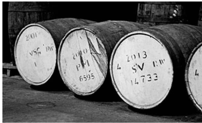
Coded casks indicate which still made the rum: VSG (Versailles), PM (Port Mourant) and SV (Savalle).
