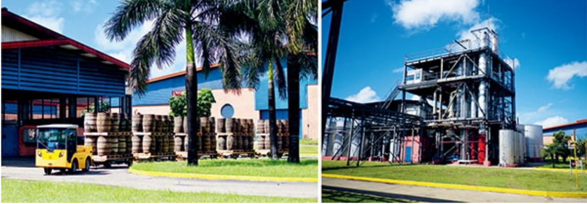
The barrel bus at Havana Club's San Jose distillery (below left) and a number of column stills at work (below right). Cuban-style rum is a blend of column-still distillates.
