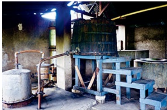
The wooden vat is both a partial condenser and a wine pre-heater.
