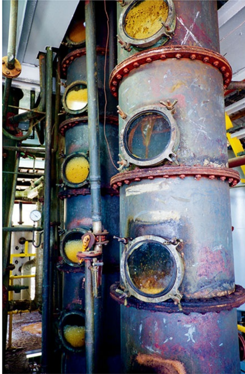
The copper portholes on the Antigua Distillery's beautiful column still offer a striking perspective of alcohol being stripped from molasses wine.
