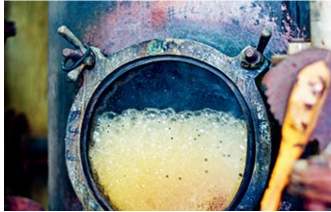
Fermented molasses bubbling through one of the plates on the column still at Antigua Distillers.
