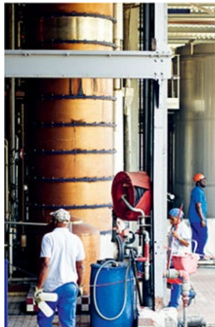
The wider the column, the higher the potential throughput. The more plates the column has, the greater the purity of spirit.
