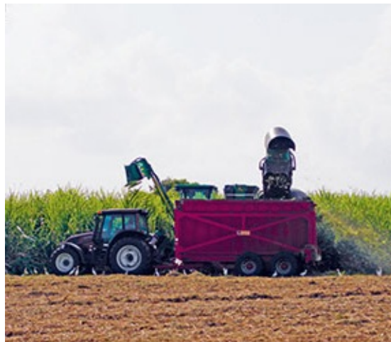
The cane cutter ploughs through the cane, and loads the cut stems into a tractor-drawn trailer. Most of the world's sugarcane is harvested in this manner.
