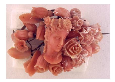
**Figure 7.** A coral brooch and ornaments of cellulose nitrate were stored in an oak barrel for many years causing white corrosion of cellulose acetate-nitrate.<sup>19</sup>
