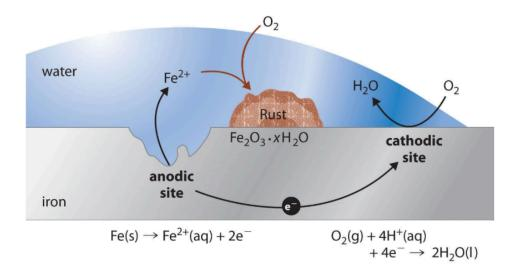
**Figure 5.** The corrosion of iron in the presence of oxygen and water with the anodic and cathodic sites on the surface of the metal indicated.<sup>23</sup>
