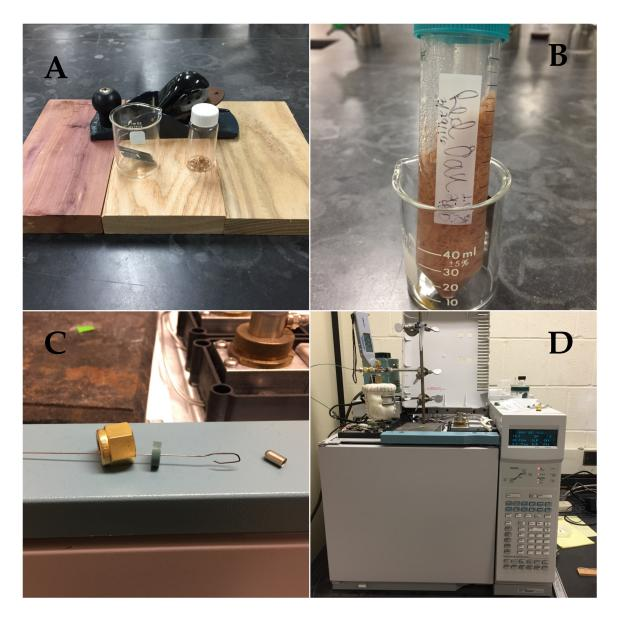
**Figure 10.** (A) Wood shaving setup including razor for fine shaving of samples. (B) Titration preparation of 2 grams of red oak wood in 20 mL of deionized water. (C) Homemade EGA cup and hook for sample injections in the oven inlet. (D) Agilent Technologies 6890N GC-FID equipped with a homemade EGA oven inlet.
