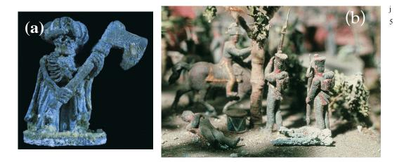
**Figure 8.** (a) A lead statue heavily damaged by acetic acid. (b) Figurines have undergone corrosion as a result of acetic acid from the wooden display board.<sup>7</sup>
