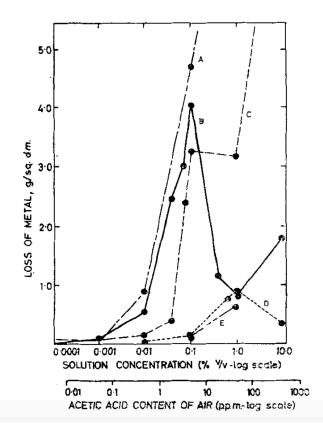
**Figure 9.** The effect of acetic acid concentration in ppm on metals from a study on corrosion of metals by acid vapors from woods by Clarke and Longhurst. (A) Steel, (B) Zinc, (C) Cadmium, (D) Copper, (E) Brass.<sup>24</sup>
