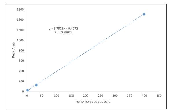
Figure 11. A calibration curve of nanomoles of acetic acid versus peak area attained from evolved gas analysis.
