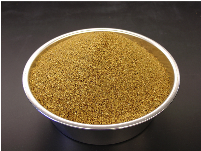
FIGURE 12.31 Distillers' dried grains with solubles (DDGS) is the primary coproduct produced by fuel ethanol manufacturing plants, and consists of all nonfermented nutrients in the cereal grain (typically concentrated by a factor of 3× due to yeast metabolism). Based, in part, on Rosentrater, K.A. 2011a. Overview of fuel ethanol production and distillers grains (Chapter 2). In: Liu, K., Rosentrater, K.A. (Eds.), Distillers Grains: Production, Processing, and Utilization. CRC Press, Boca Raton, FL, USA.
