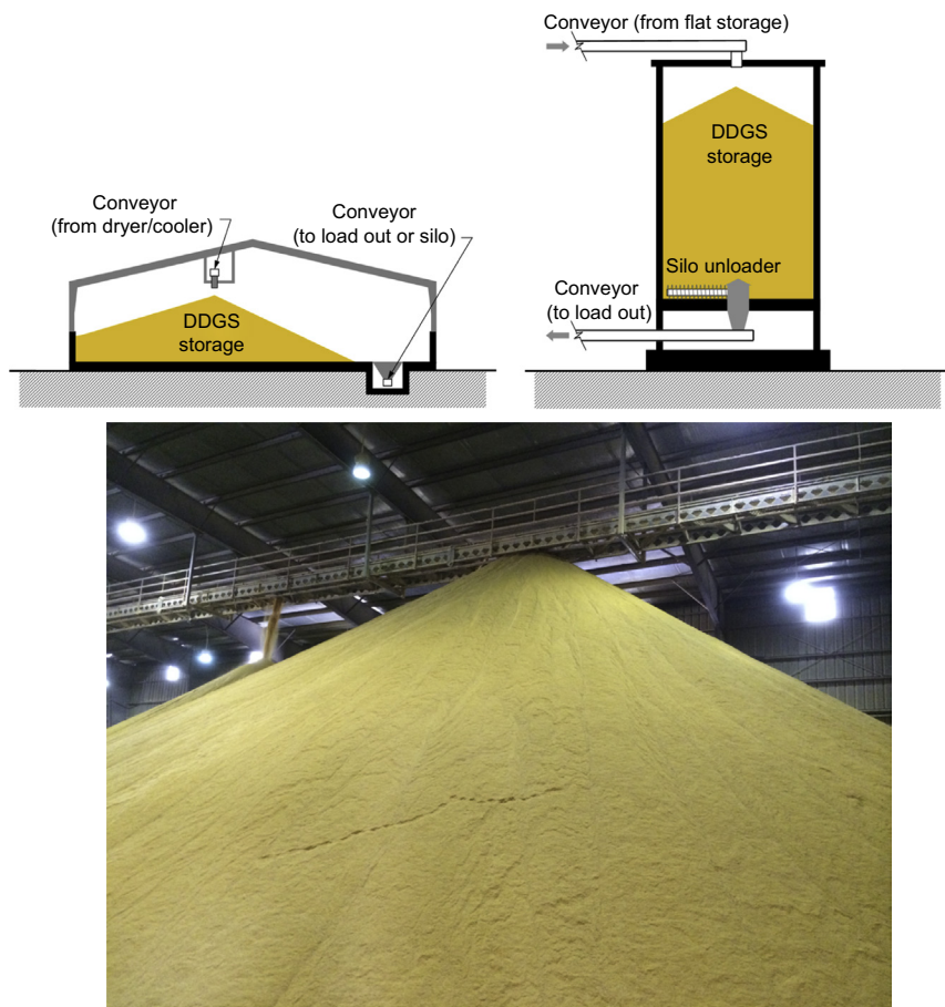
FIGURE 12.32 Distillers' dried grains with solubles (DDGS) storage typically occurs in either steel-sided flat storage buildings or concrete silos. Based, in part, on Rosentrater, K.A., 2011b. Manufacturing of fuel ethanol and distillers grains – current and evolving processes (Chapter 5). In: Liu, K., Rosentrater, K.A. (Eds.), Distillers Grains: Production, Processing, and Utilization . CRC Press, Boca Raton, FL, USA.
