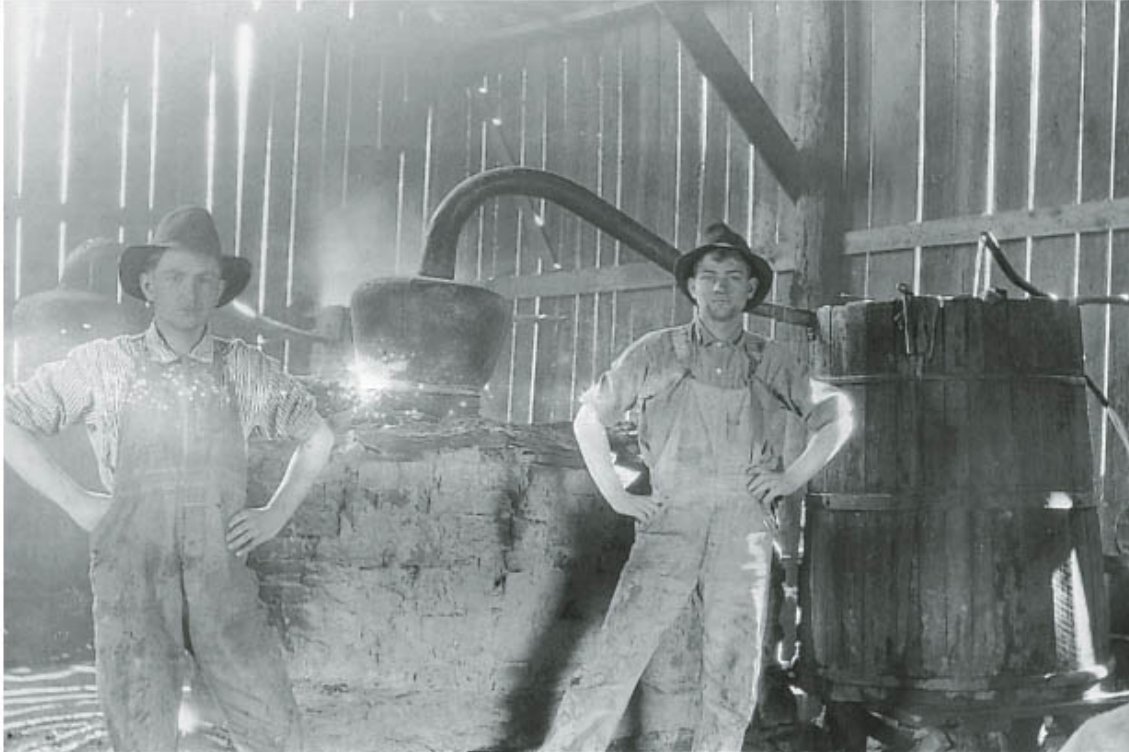
Pot stills at the Harlan Distillery in Monroe County, Kentucky, 1918. This photograph could have been taken in 1818, as the technology remained the same a century later. (Courtesy United Distillers Archive)
