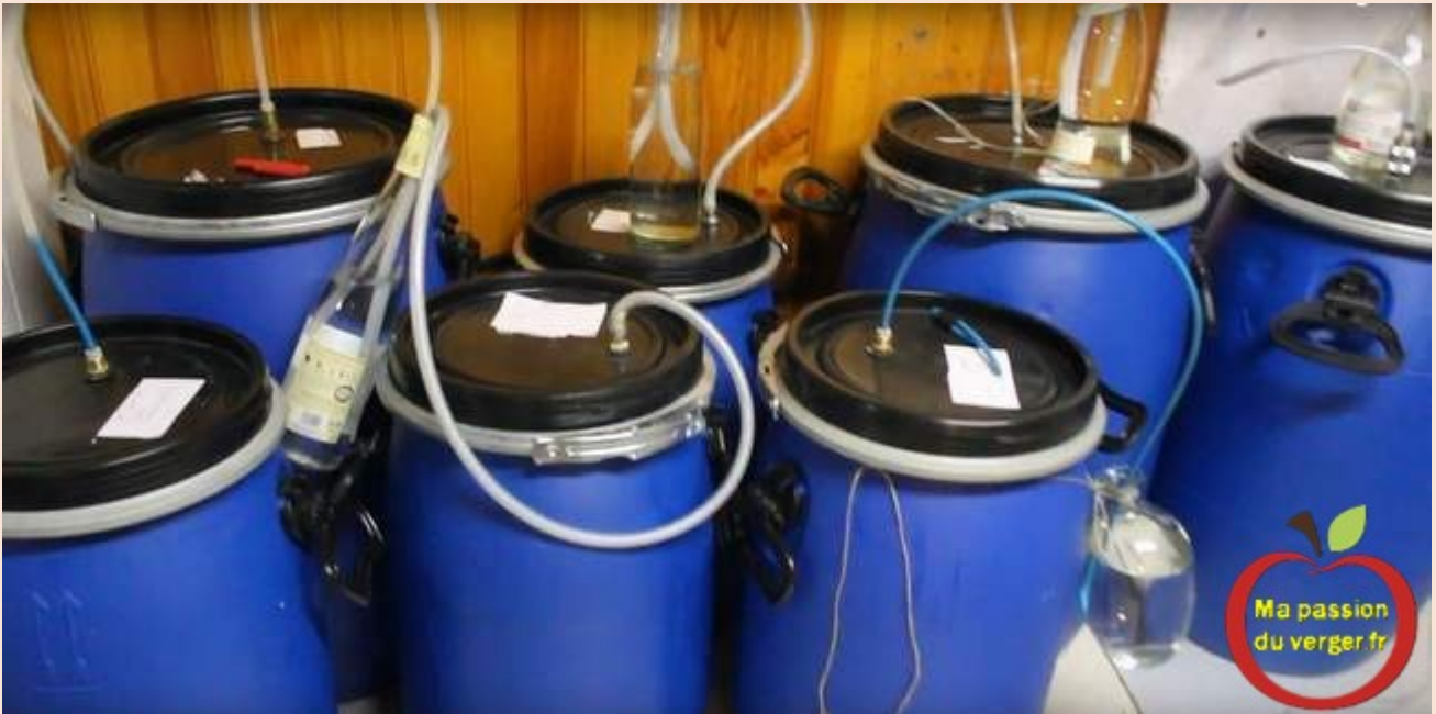
Homemade bubbler manufacture, based on a photo by Jean-Luc Lett (Arboriculteurs Hambach) Just attach a pipe with a fitting on the cover and put it in a bottle of water.
