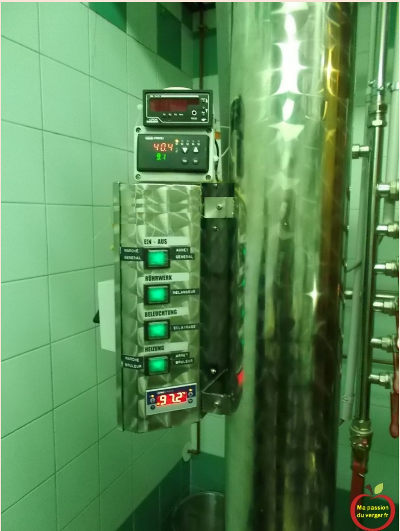
When the alcohol vapor temperature display shows 42 ° the burner must be lowered.
