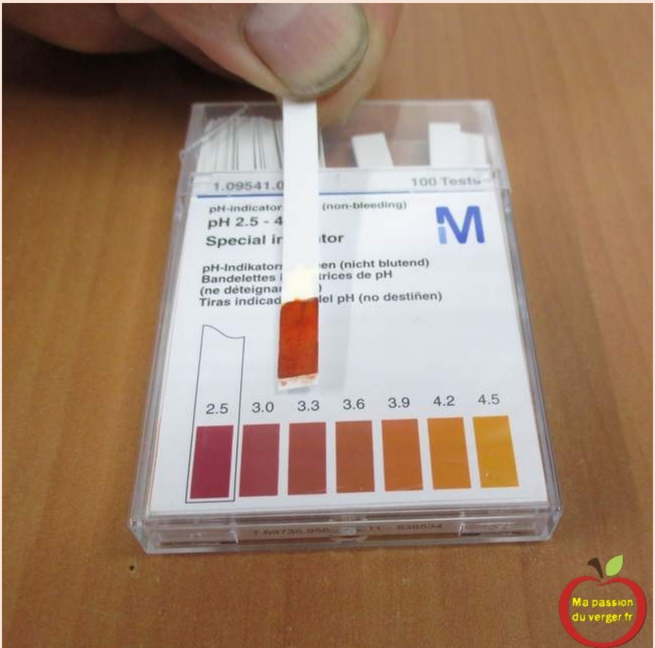
Measure the pH of your must using a test strip. Soak in the mash for at least 2 seconds. Thanks to the color scale supplied with it, you can quickly recognize the exact pH value of your fruit puree. (Simaco strip)
