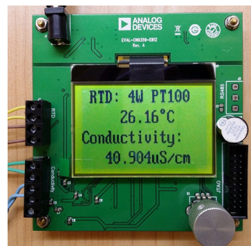
Figure 12. Photo of an EVAL-CN0359-EB1Z board showing the home screen in measurement mode.
