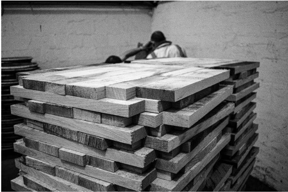
Figure 6b Finished heading
