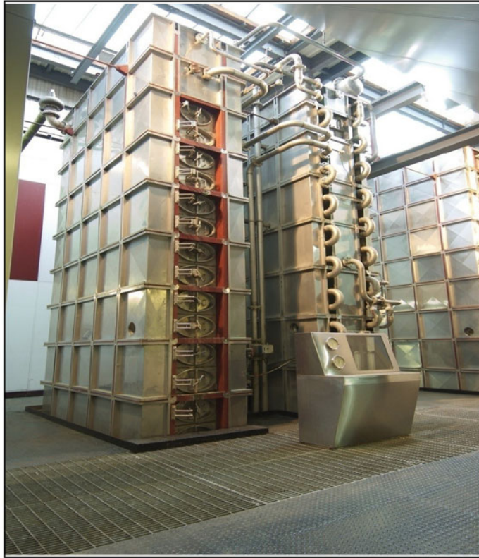
Figure 67 – Modern Coffey Still (North British Distillery)
