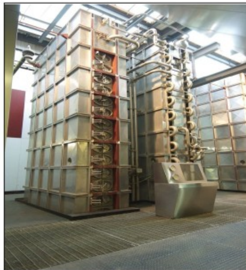
Figure 67 – Modern Coffey Still (North British Distillery)
