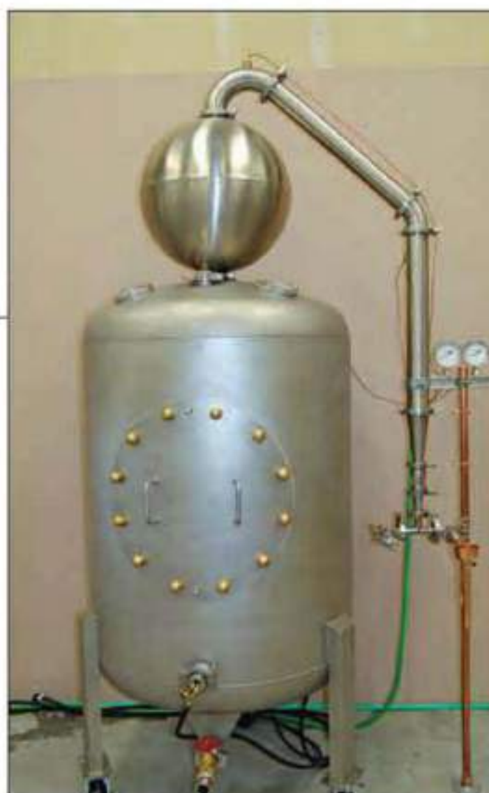
This alambic still was custom-built by Dynamic Alambic by reconfiguring a Grundig beer tank.
