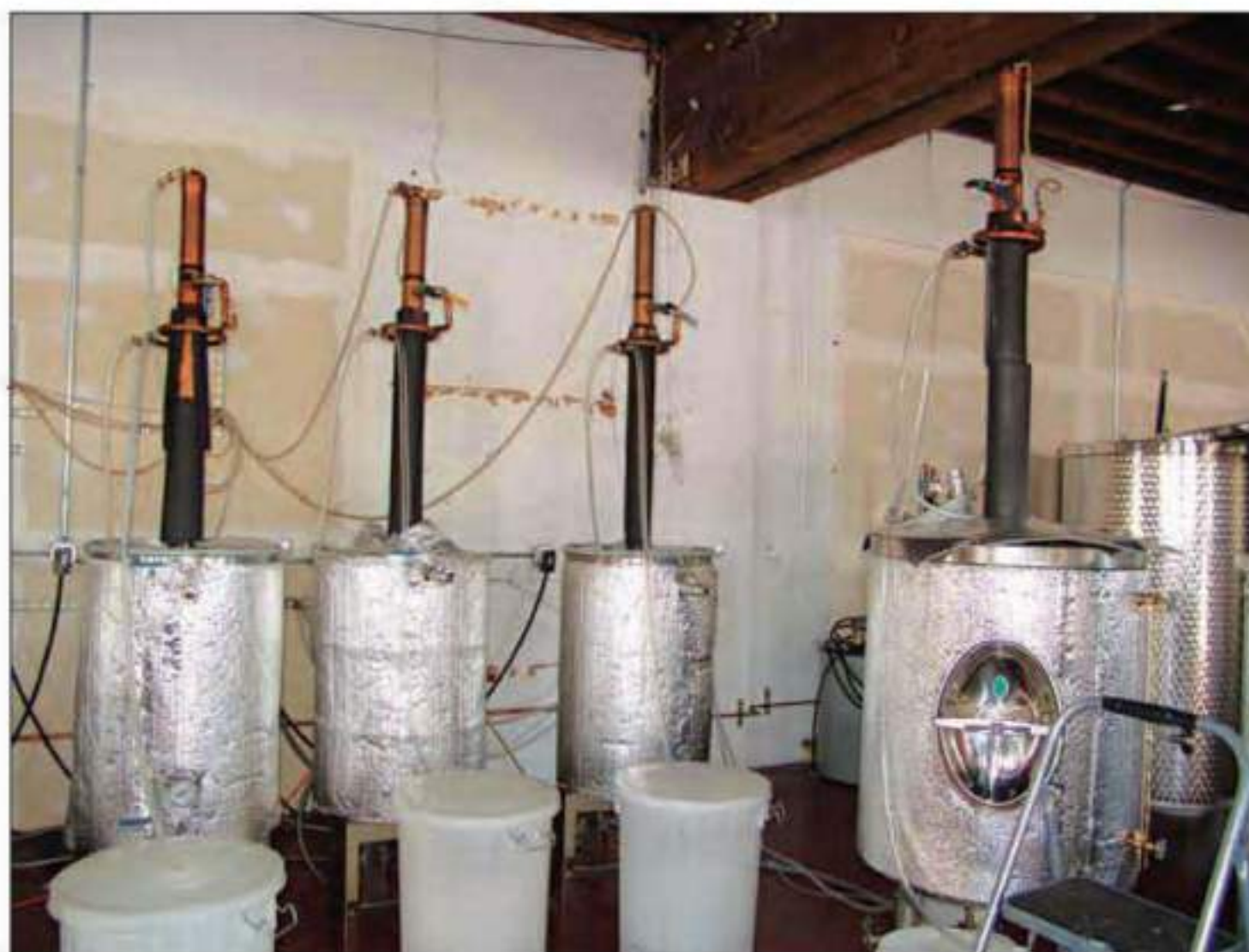
Three stripping stills and a spirit still made from stainless steel drums at the New Deal Distillery
