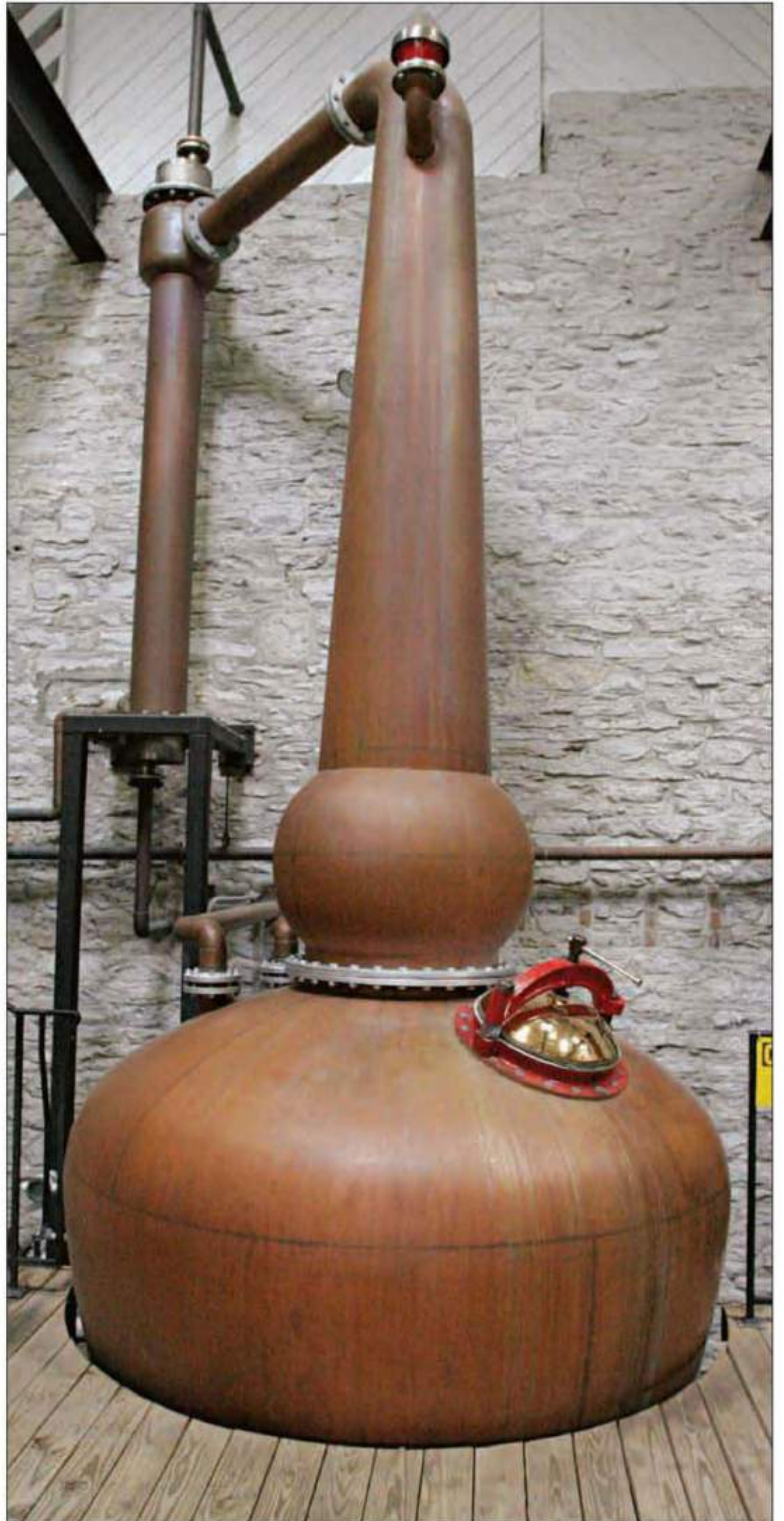
A gooseneck still clearly showing the lyne arm at Woodford Reserve Distillery
