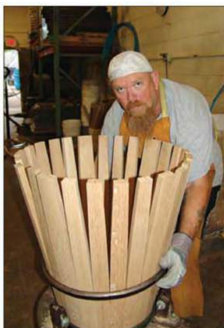
A cooper forms a barrel before attaching hoops around the outside.
