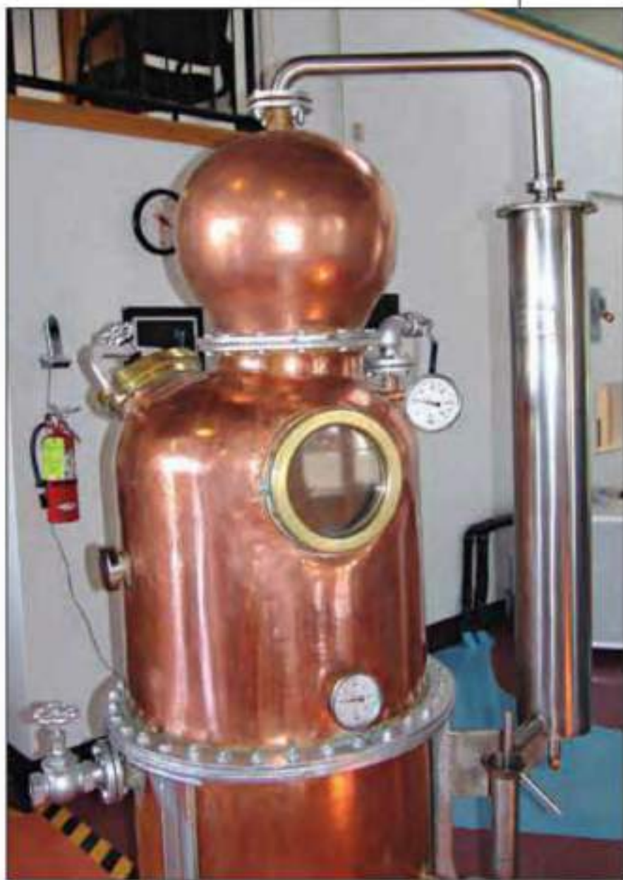
Artisan pot still: the shape of the helmet "head" of the still influences the flavor of the distillate.
