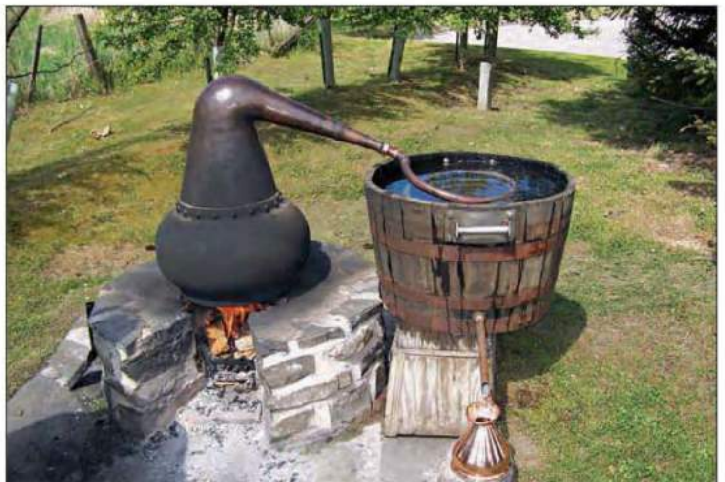
A small pot still, similar to many moonshine stills, is in operation for tourists to see at the Glenmorangie Distillery, Scotland.
