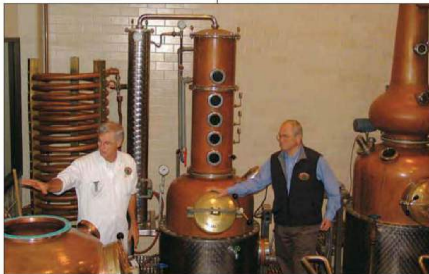
Fritz Maytag, right, at Anchor Distilling. With a small overhead crane, Anchor Distilling can interchange the columns of their three stills.
