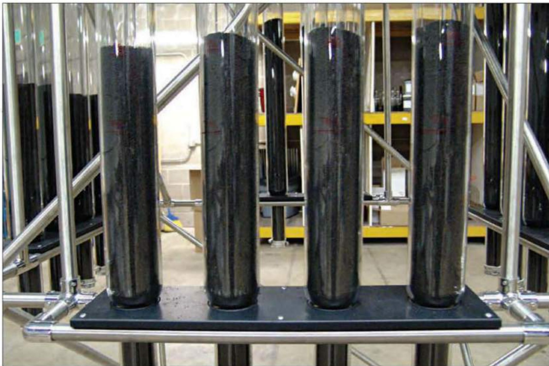
Charcoal filtration used in making vodka at Colorado Pure Distilling
