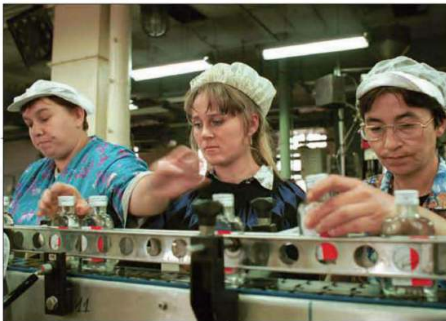
Putting labels over the caps of freshly filled bottles of Prezydent Vodka at Polmos Lodz in Lodz, Poland
