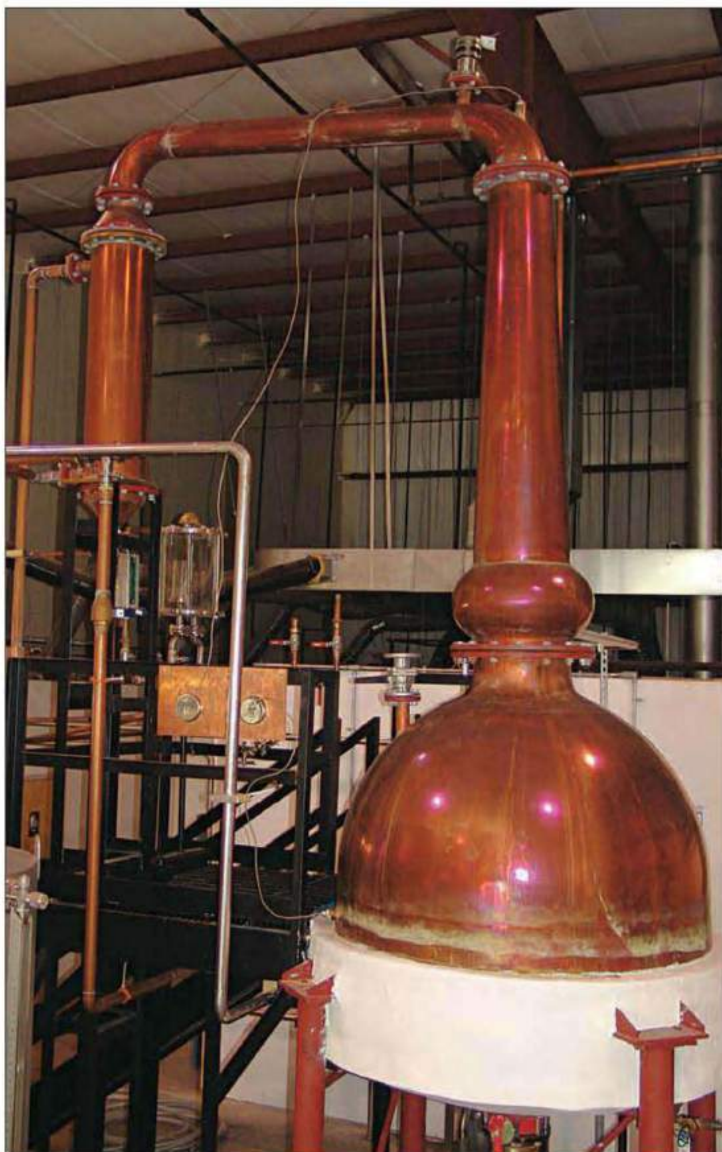
A gooseneck still is used to produce Bluecoat Gin.
