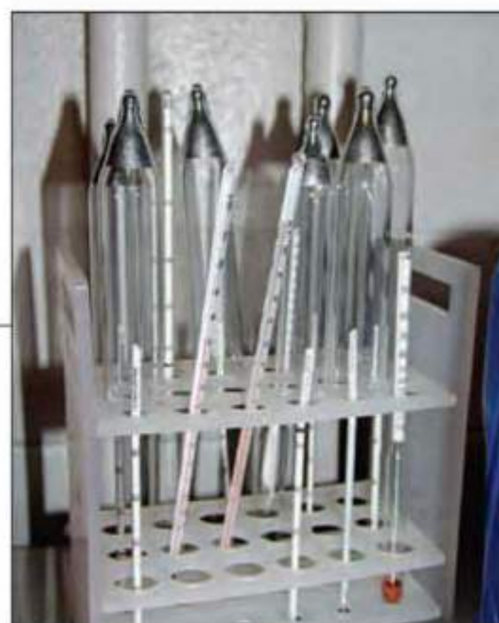
Hydrometers for measuring alcohol content of distillates
