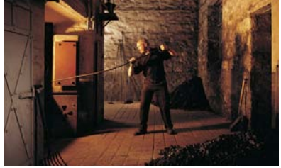
The kilns at Balvenie Distillery are fired up with the addition of peat to create a distinctive, phenolic characteristic in the whisky.
