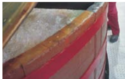
At Aberfeldy , there are eight large washbacks made of Siberian larch, with two additional state-of-the-art stainless-steel washbacks nearby.
