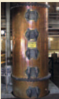
A Coffey still is able to work continuously rather than in batches, as with a pot still.
