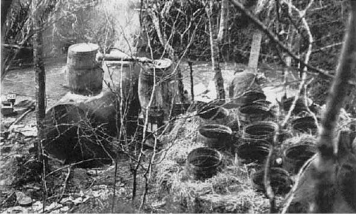
Fifty-gallon wooden barrel fermenters at a stream-side still site. Bureau of Alcohol, Tobacco, and Firearms, U.S. Department of Treasury.
