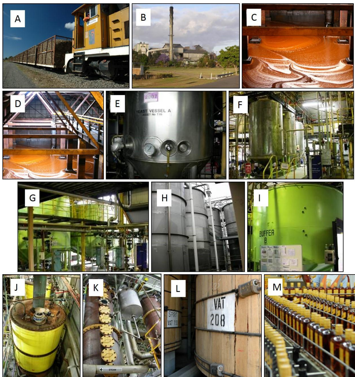
Figure 3.2 Process steps at the Bundaberg Distilling Company. (a) Cane harvest, (b) sugar mill, (c) molasses, (d) molasses storage tank, (e) yeast vessel A, (f) yeast vessels, (g) small fermenters, (h) large stainless steel fermenters, (i) buffer tank, (j) pot still, (k) continuous still, (l) maturation vat, (m) bottling.
