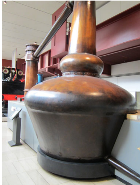
Figure 1. A copper still manufactured in Scotland for the Glenfiddich distillery in the 1960s and now on display in National Museums Scotland, Edinburgh. In size and design, it is similar to the vessel produced by Forbes for Barham in 1775.
